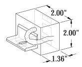
Mini Multi-Hanger Inline Coil 120 VAC = P/N 6-42-115 240 VAC = P/N 6-42-128
