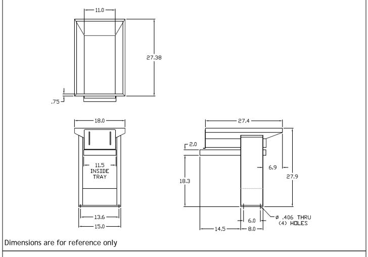
Optional: Photoelectric Parts Level Sensor P/N 111-000-0521
