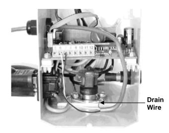
Example of a "drain" wire termination
