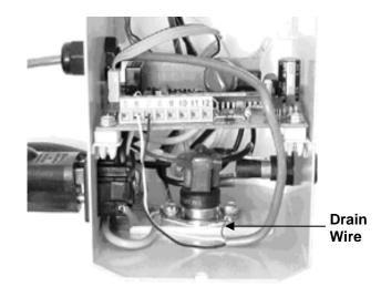
Example of a "drain" wire termination
