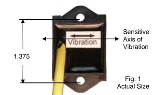
**A. ORIENT THE SENSOR** so that its sensitive axis is in the same direction as the vibration of the feeder. The arrow in figure 1 shows the sensor's sensitive axis. Align the sensitive axis of the sensor in the same direction as the vibration (see figure 2). The sensor must be oriented correctly for proper operation.
