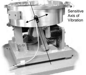
Fig. 2 The arrow shows the direction of vibration which is at a right angle to the spring pack. FC-200 Set Up.docx 3/24/2017 Page 5
