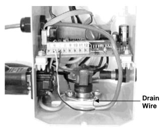
Example of a "drain" wire termination
