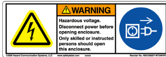
Figure 1 – Warning label installed on the control
