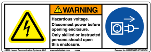
Figure 1 – Warning label installed on the control
